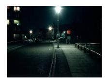
This is a typical side road with a 80watt mercury vapour lamp. These lamps last a very long time, produce a white light but have poor performance in terms of lumens per watt
